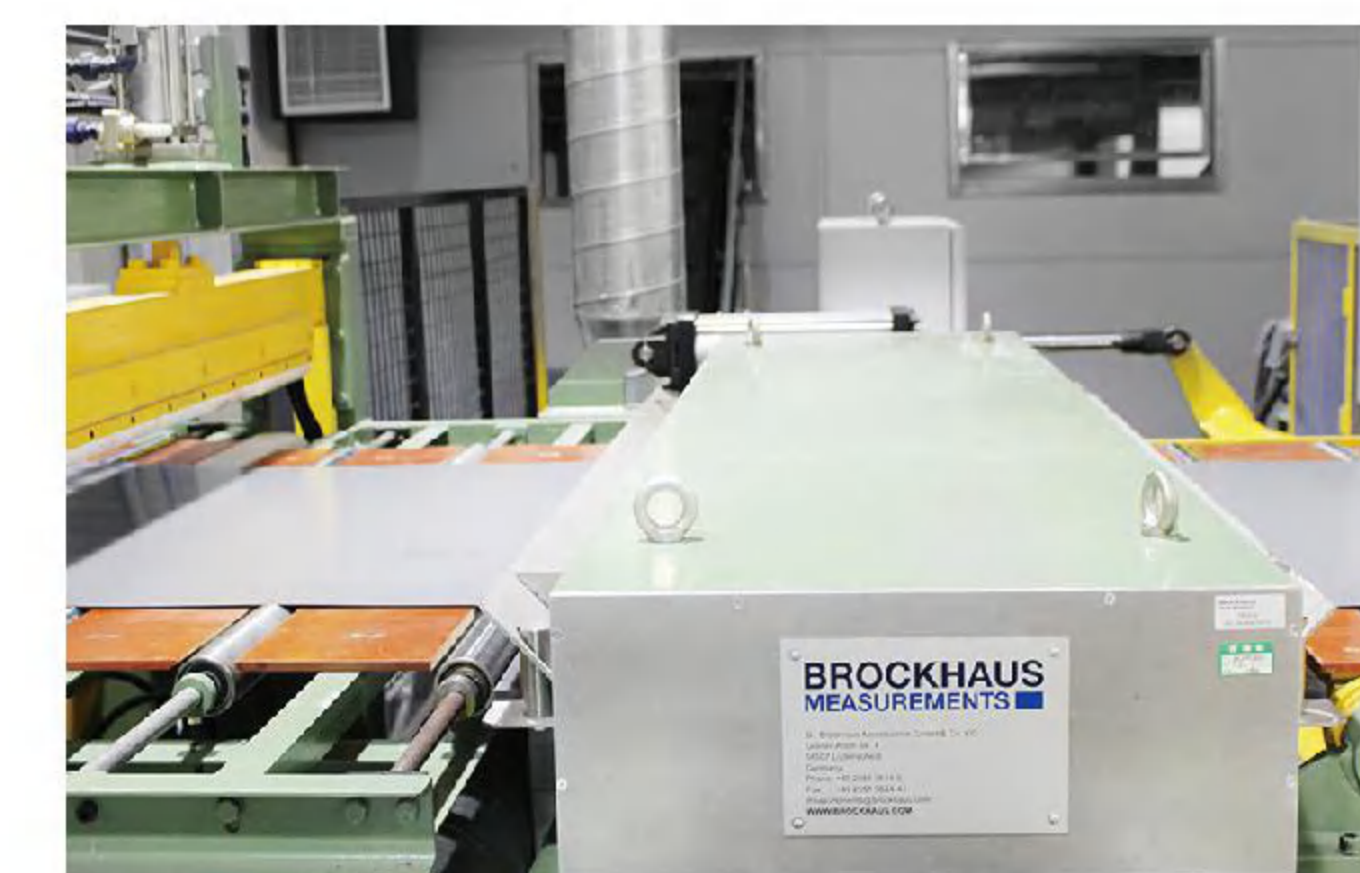
EBA - Continuous Inline Magnetic Properties Measurement System
